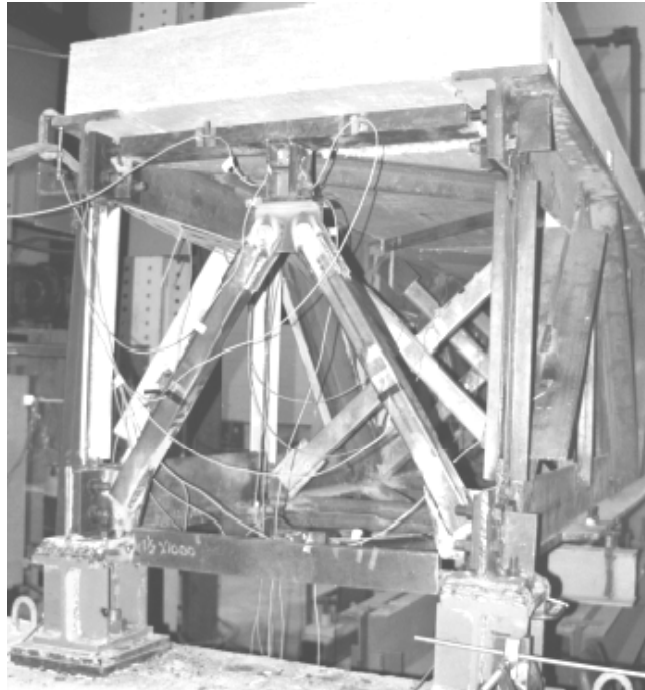
Figure 3. Steel ductile retrofit at the end panel
